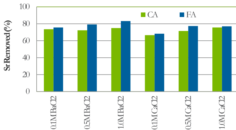
Figure 6. Desorption of Sr 2+ from coarse and fine aggregates (CA and FA, respectively) of concrete using Ba and Ca salts. V/m= 1.
